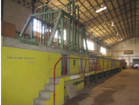
A Wave Flume for 2-D tests, with active wave absorption.
