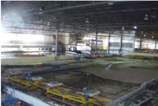
A Wave Basin for 3-D tests.
