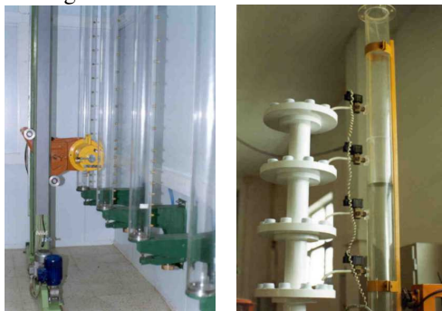
Set-up for consolidation tests, settling column
