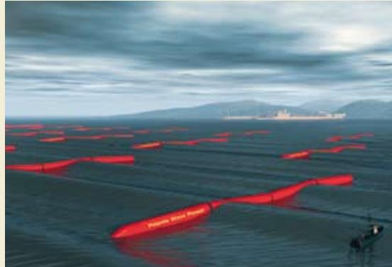
7.12 c > The Pelamis wave energy transformer floats on the ocean like a giant sea snake. It consists of several segments which move against each other and build up hydraulic pressure. This in turn drives a turbine. A new Pelamis generation is currently under construction.
